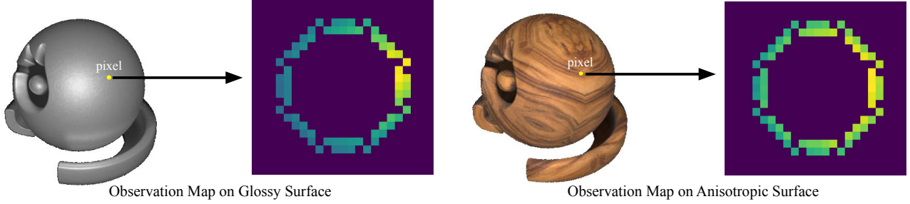
Figure 4. Illustration of observation maps corresponding to the pixel marked with yellow color. Each element of the observation map corresponds to the image intensity measured under different lighting. For a glossy surface, an observation map clearly reveals the specular region, providing strong cues for reliable prediction of surface normals. On the other hand, anisotropic surfaces exhibit more irregular distribution w.r.t. light source directions, which makes it difficult to predict surface normals reliably.
